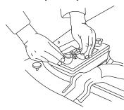
**11**. Ground amplifier to chassis of vehicle; connect the terminal provided to the 10ga black wire from furnished wiring harness. A good ground is as important as the power connection. The ground should be as short as possible and the contact point should be free of paint and debris.
